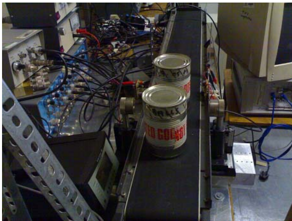
Fig.8 A scanning system for canned products on a conveyor belt.
